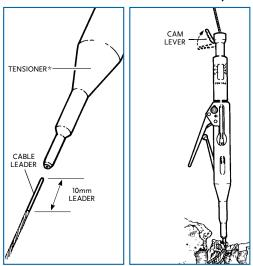
To remove cable slack, hold bottom shaft of Tensioner while extending upper shaft of Tensioner\*.
