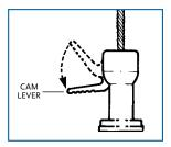
To secure Integral Crimp\* onto cable, position Crimper\* jaws around Integral Crimp\* and squeeze Crimper Handles once until the Crimper Stops touch.
